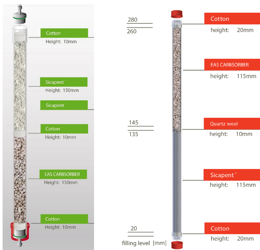
Figure 1: Schematic figure of the absorption tube filling of a rapid MAX N exceed (left) and a vario EL cube (O-mode) (right).
